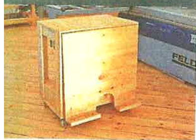
To lift 4x8' sheet goods onto the saw table, Bill loads the material on the side of this mobile bench, raises the hinged side, and then slides the sheet across the bench and onto the saw.
